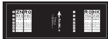
Test No. 8, SA-BRL-4 —Visual Acuity Results calibrated at 20/20, 20/30, 20/40, 20/50, 20/70, 20/100 and 20/200. Tests can be administered binocularly or with either eye occluded.
